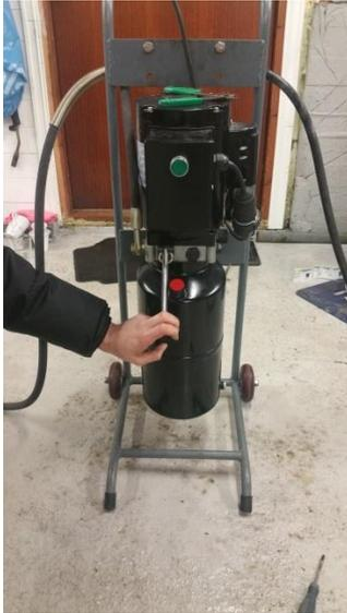
When you have completed the bleed process the lifting arms should be on the ground! And **REMEMBER** to fasten the Bleed screw before this next step!!!
