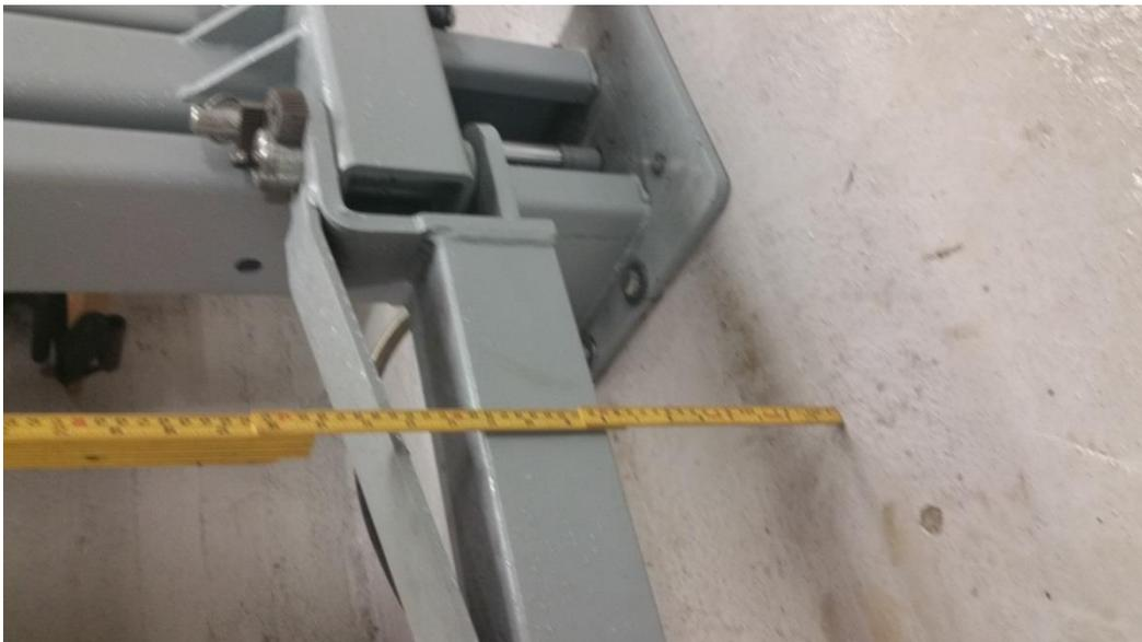
4. Open the cylinder bleed screw. And let the lifting arms lower to the ground. (Note! If you fully open the screw the lifting arms will fall down, keep in mind were you have your feet)
