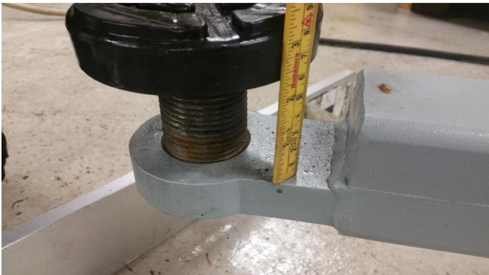
6. Level the lifting arms by bleeding the cylinder on the highest side until the lift is leveled.
