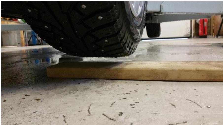
Lift the car 5 cm over the floor. Make sure the locks on the inner arms are engaged. Make the car sit for a few minutes, while you make sure there are no leaks, and that the car does not lower it self
